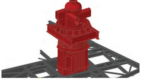
Cyclone 3-D model screenshots illustrating a removal lift.
